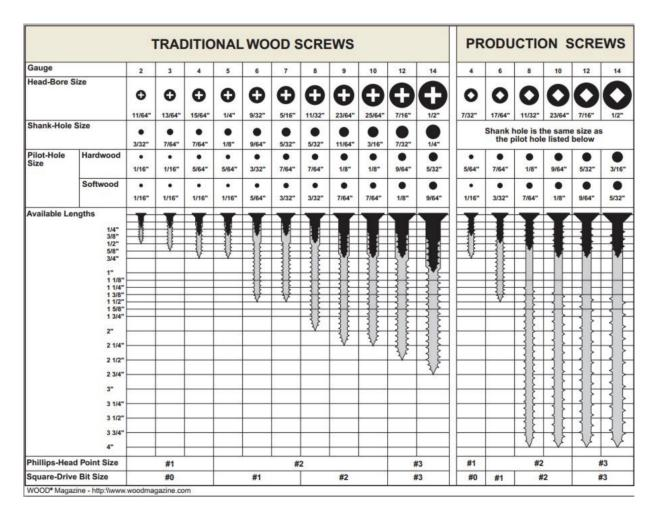
prevents the wood from splitting out and the screw from being bound up and then breaking. Shown below is a chart that has the most common wood screw sizes and lengths.
