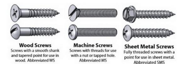
Sheet metal screws like wood screws fasten directly into the material you are fastening.
